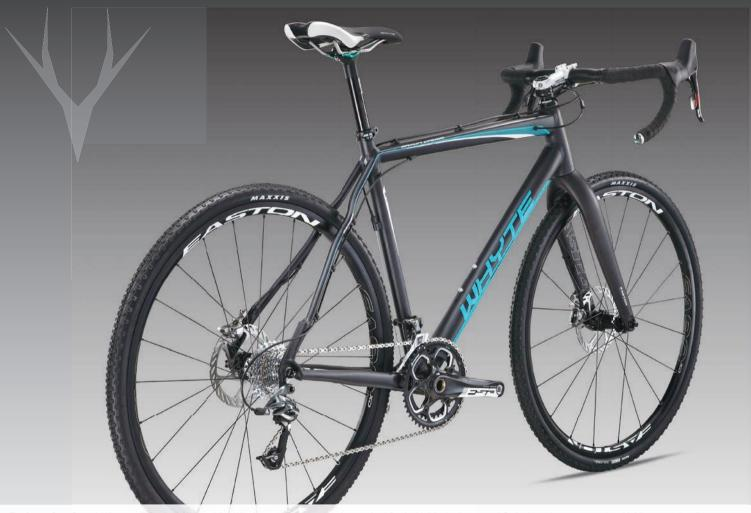
■ The Saxon Cross Team is Whyte's off the shelf CX race bike. Whether round the local park or on the 3 Peaks this bike is all you need. Trail oriented geometry makes this bike exceptionally competent and controllable off-road. ■ SRAM's Force 11 speed group combined with the new RED22 levers give you the world's first fully hydraulic disk road brakes. ■ Easton's straight bladed EA990 XD carbon fork with its tapered steerer tube gives this bike great front end stiffness and steering precision.
