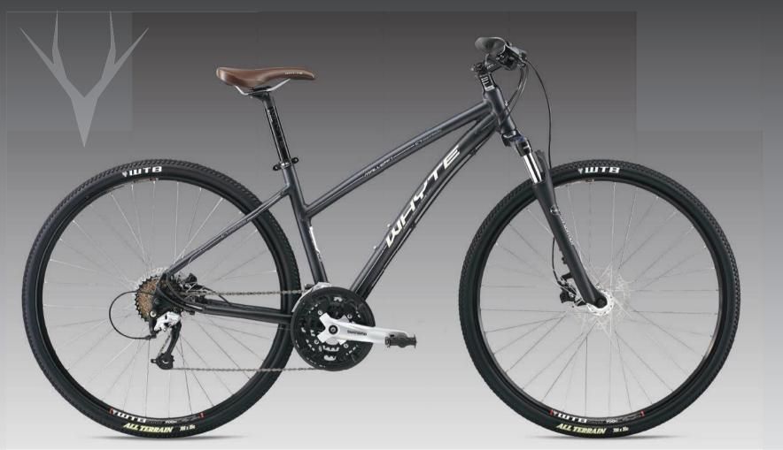
■ All the same key design features as the unisex version, with the added benefit of a partially dropped top tube. This increases standover height, while still keeping enough room inside the frame to comfortably fit a water bottle. ■ Another benefit of the partially dropped tube is the maintained stiffness of the frame (fully dropped top tube frames are flexi and offer less steering control).
