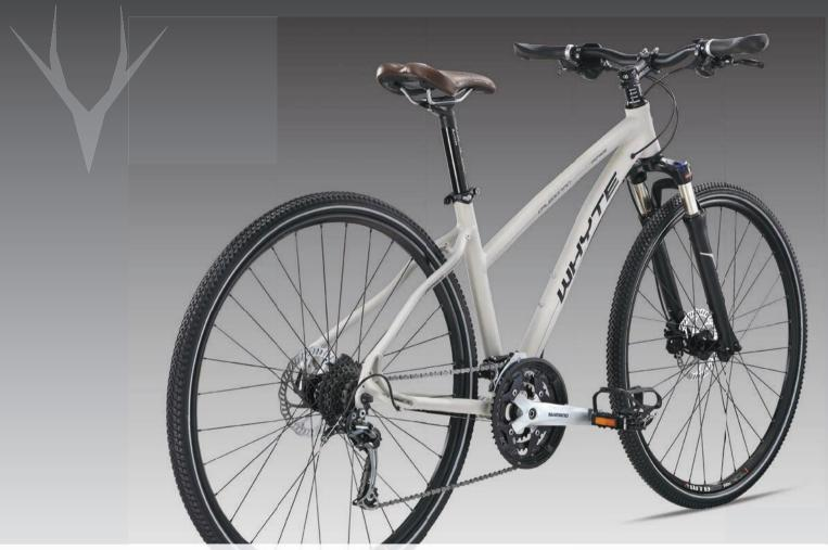
■ All the same key design features as the men's version, with the added benefit of a partially dropped top tube. This increases standover height, while still keeping enough room inside the frame to comfortably fit a water bottle. ■ Another benefit of the partially dropped tube is the maintained stiffness of the frame (fully dropped top tube frames are flexi and offer less steering control).
